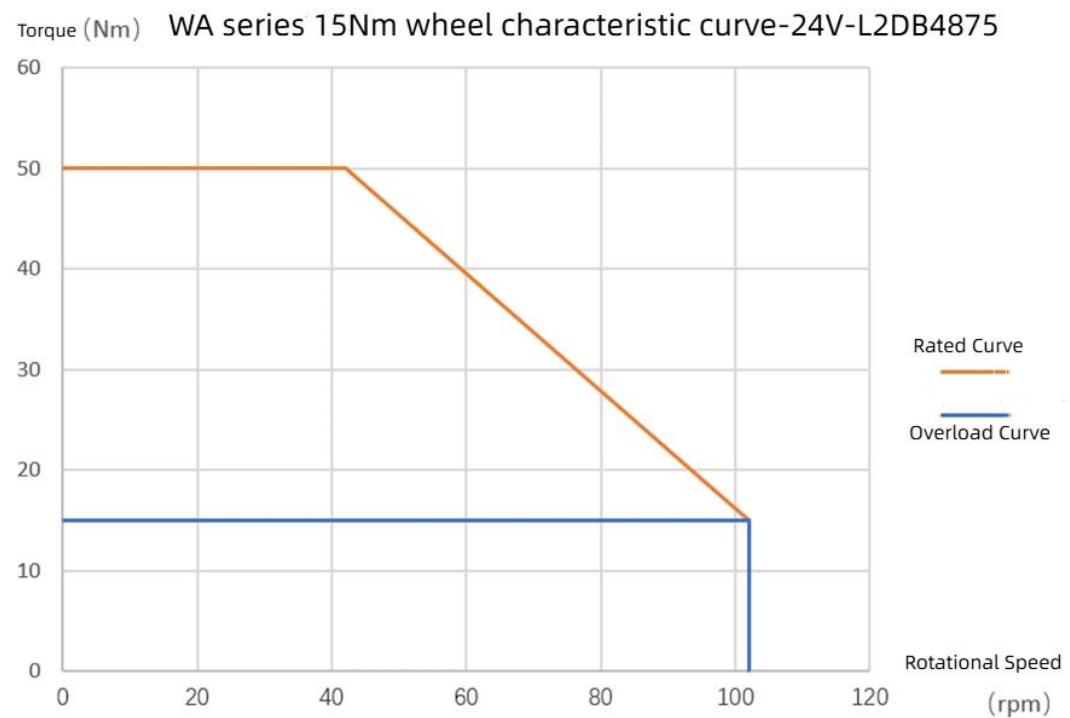
Figure 2.2.2-4 24V characteristic curve of the WA series L2DB4875 15Nm hub motor
